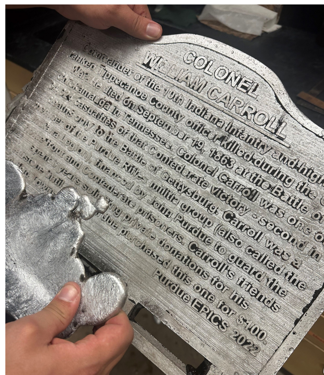
Successful casting of the plaque directly after being removed from the sand mold.
