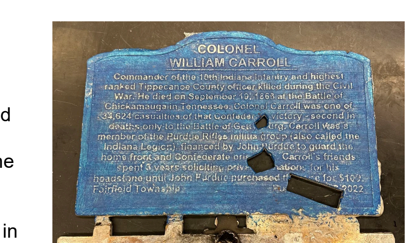
Third casting showing the gating system still attached and the areas in which sand fell into the mold cavity. This casting was painted blue and then sanded to test if the lettering was more visible with the new pattern.
